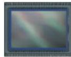
APS-C size sensor: approx. 22 x 15mm
