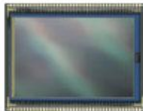
APS-H size sensor: approx. 29 x 19mm
