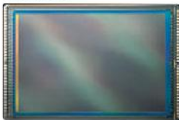
35mm full-frame sensor: approx. 36 x 24mm
